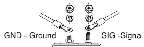
3. Connect the end of the black ground wire to ground (GND). Connect the signal wire (SIG) to the signal wire of the gauge. Your installation is now complete.
