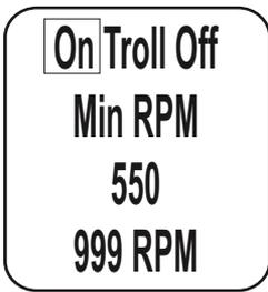
Once the troll function is “ON”, press the “Up” or “Down” buttons to change the troll setting.
