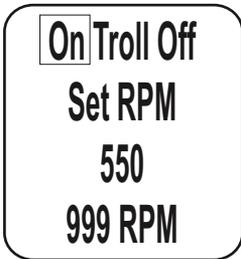
The troll control function has two modes of operation, “RPM mode” and “Speed mode”. Press and hold both “Up” and “Down” buttons in the, Troll mode, to switch between the two modes.
