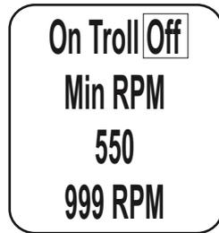
Press “Mode” to turn the troll control function “ON” and “OFF”.
