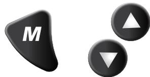
In the "Normal" mode, pressing the "Down" or "Up" buttons causes the display to cycle between the available screens (see Figure 2, page 11).
