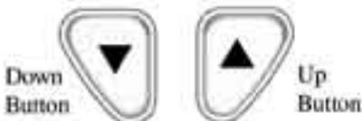
When finished, press the ‘M’ mode button to exit the adjustment screen. The operator has the option of saving or canceling the adjustment procedure. The options can be selected using the “UP” or “DOWN” push buttons. To save the calibration setting, press and hold the ‘M’ mode button for 2 seconds when the display shows “SAVE”.
