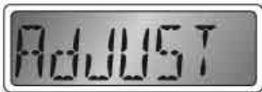
Run the boat at a constant 30 MPH as measured by the GPS or radar. Adjust the speedometer pointer by pressing the “UP” or “DOWN” arrows until the speedometer matches the GPS or radar speed.
