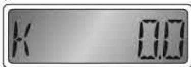
Pressing the “Up” or “Down” buttons will change the keel offset setting.
