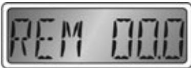
In normal use, the amount of fuel in the fuel tank is adjusted manually when the fuel tank is filled so that this display shows the total amount of fuel in the tank. The “Trip Fuel Consumed” is then reset to zero. As fuel is used (displayed in the “Trip Fuel
