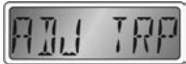
Pressing the “Mode” button for more than one second will cause the display to go into the Trip Fuel Consumed adjustment menu.
