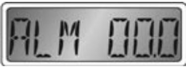
When the “Fuel Remaining” reaches this amount, the “Low Fuel” alarm will sound and a warning LED will flash in the display.
