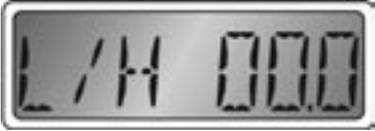
Leaving the display in one of the items above while the “Mode” button is pressed and held for more than one second will save the selected units.
