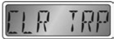
Pressing the “Mode” button for more than one second while the display shows “CLR TRP” will clear the trip amount and set the menu back to the Trip Fuel Consumed function.
