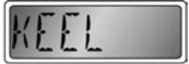
Pressing the “Up” or “Down” button changes the setting for the Keel Offset.
