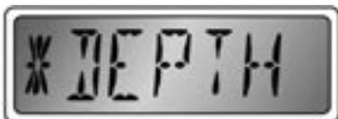
The depth can be displayed in feet, meters, or fathoms. Audible and visual alarms can be set to warn of shallow or deep water conditions. A “keel offset” setting allows the operator to adjust for the difference in the location of the Depth Sounder transducer compared to the deepest part of the boats hull.
