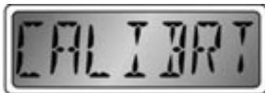
This menu item is used to simultaneously adjust the calibration of the Speedometer and the Trip Log. Two methods of calibration are possible. These methods will be discussed in the Calibration Section.
