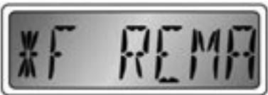
The Fuel Remaining display shows the amount of fuel remaining in G or L.
