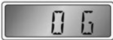
This gauge is useful for keeping track of fuel usage over a longer period of time or distance than the Fuel Used gauge. The display is based on the fuel flow system and therefore filling the fuel tank
