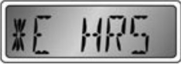
The Engine Hours display shows the number of hours the engine has been operated (Hr). The reading is based on a signal being received at the tachometer input to indicate that the engine is running. Units are displayed as:
