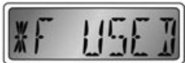
The Fuel Used display shows the amount of fuel used since the gauge was reset. The display is based on the fuel flow system and therefore filling the fuel tank will not disturb the reading.
