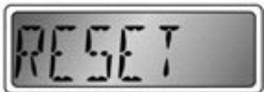
Pressing the “Up” and “Down” button resets the Fuel Used gauge to zero.
