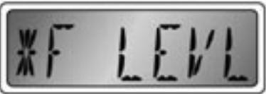
The Fuel Level display shows the amount of fuel in the fuel tank in percent of full (PC).
