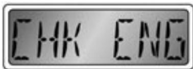
If a check engine warning is displayed when the engine is running, the words “CHK ENG” will be indicated on the LCD screen. You must stop the engine to retrieve the “flash” code that designates which problem has occurred. You must return to engine idle speed and either pull the emergency stop switch to stop the engine (but leave the ignition key in the on position) or turn the key switch off to stop the engine, then turn it back on (do not restart the engine).
