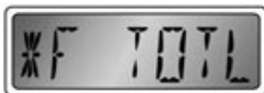
The Total Fuel Used display shows the amount of fuel used since the Total Fuel Used gauge was reset.
