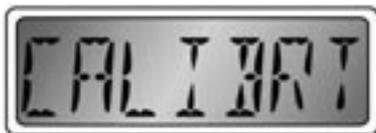
If you know “exactly” how much fuel you have used since the Fuel Used gauge was reset you can adjust the amount and, therefore, the Fuel Flow sensor calibration in this “setting” menu.
