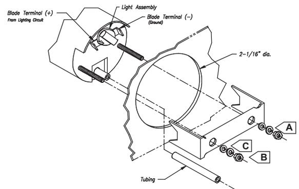
**NOTE:** To change the light bulb, twist out black socket assembly one-eighth turn counterclockwise until it pops out. Bulb pulls straight out of assembly. It is a GE No. 161 instrument lamp.
