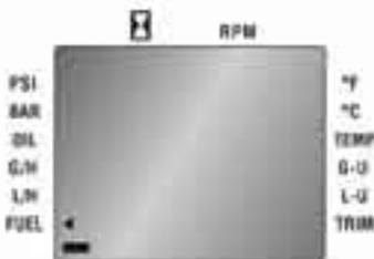
This function provides a continuous monitor of fuel level. Used in conjunction with the calibrated Fuel Remaining in Tank function and alarm, very accurate monitoring of fuel level can be obtained.
