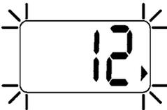
Use the ▲ and ▼ keys to select the desired alarm value. Press and hold both keys for one second to save this new value to memory and to exit this function. The display will indicate **ALr** and then the new value.
