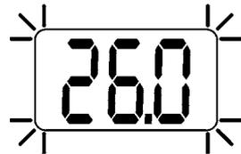
Use the ▲ and ▼ keys to change the value. Press and hold both keys for one second to save this new value to memory and to exit this function. The display will indicate GAS and then the new value.
