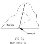
until the bottom of the paddle wheel support is parallel to the bottom of the boat with it's small "lip" hooked against the transom's bottom. (Refer to figure 1c). Tighten the two machine screws. Holding the sensor in the desired location, trace the outline of the mounting holes onto the transom. NOTE: It may be necessary in some applications to tilt the paddlewheel support deeper than parallel to increase high-speed sensitivity.
