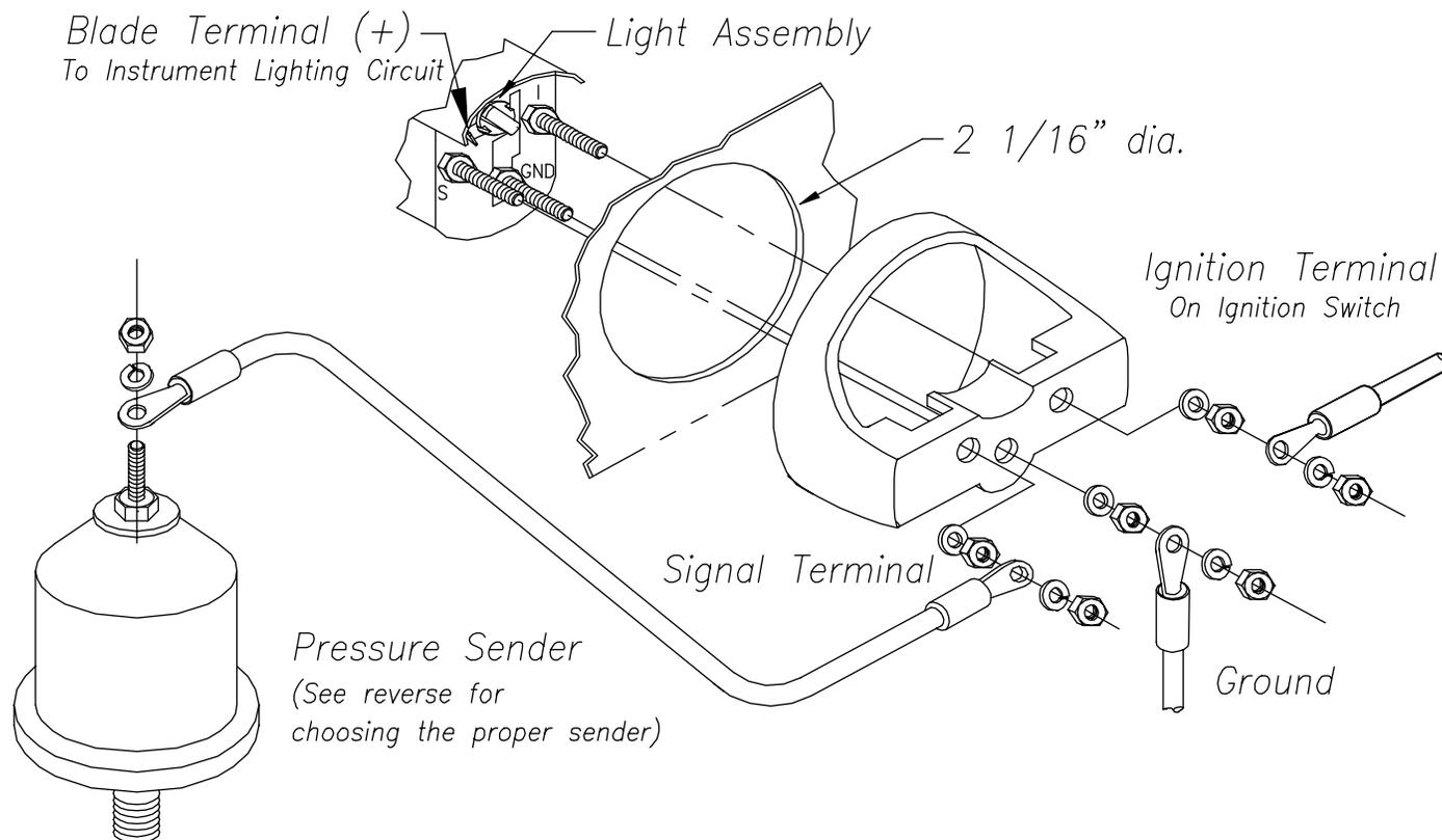
**CAUTION:** Disconnect the battery during installation. Tighten nuts on the only slightly more than you can tighten with your fingers. Six **inch-pounds** of torque is sufficient. Over tightening may result in damage to the instrument and may void your warranty. These instructions concern only fuel pressure gauge installations. **SPECIAL CAUTION** should be taken when working on or near lines that have, or have had, fuel in them.
