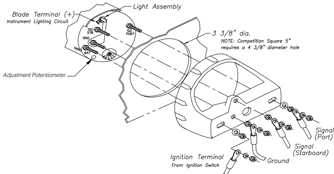
The Faria® Marine dual engine synchronizer is designed to indicate engine synchronization extremely accurately when the speeds of the two engines are compared to each other. Engine synchronization may be difficult at idle speeds. For proper operation, both engines must be of the same type, have the same number of cylinders, and have similar ignitions. Malfunctioning ignition systems or high speed “point bounce” will result in inability to sync properly.
